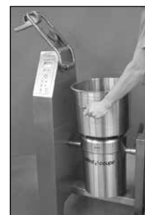
17) Put back the bowl, pouring lip on left hand side
