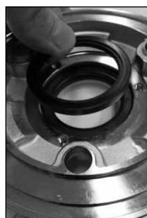
13) Put the centring ring on.
