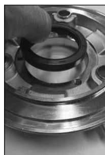
12) Put the lip seal on. Make sure it is facing the right way: groove towards the deflector.
