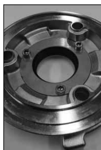
14) Put the flange and screws back on.
