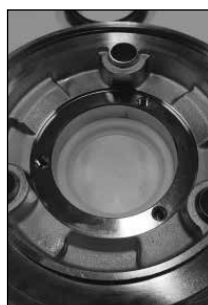
11) Check that the seal has been inserted properly.
