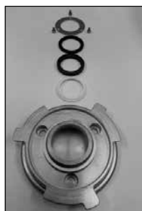
8) The assembly comprises 4 rings + 3 screws.
