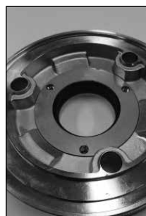
9) Remove the 3 screws and 4 rings.
