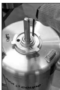
5) Remove the screws and washers.
